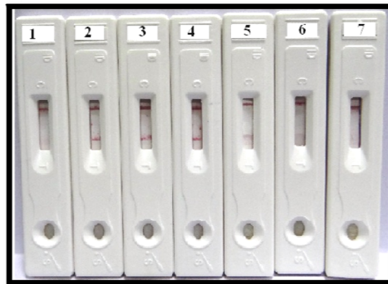
Fig. 4.11: Sensitivity determination of SEDIA device. A logarithmic dilution (1000 ng /ml to 0.01 ng/ ml) of CV and RV venoms prepared in PBS and applied on SEDIA device. Fig. (A) and (B) representing the sensitivity CV and RV respectively. Device 1: negative control, the device 2 to 7 applied from left to right with decreasing logarithmic dilutions of spiked venom samples. In both figures device 7 shown only the control line, therefore sensitivity of SEDIA device is 0.1 ng/ml.
