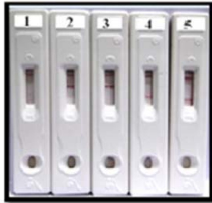
Fig. 4.12: Experimental envenomation determination by the SEDIA. The device 2 and 3 representing results of CV and the device 4 and 5 for the RV envenomation produced the red lines at test as well as control zones, while device 1 produced a red line at control zone only; confirms the efficiency of the SEDIA device to selectively detect experimental envenomation.
