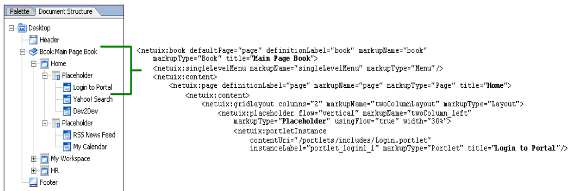
Fig: 6.4 Hirarchical Structure of Desktop Portal
