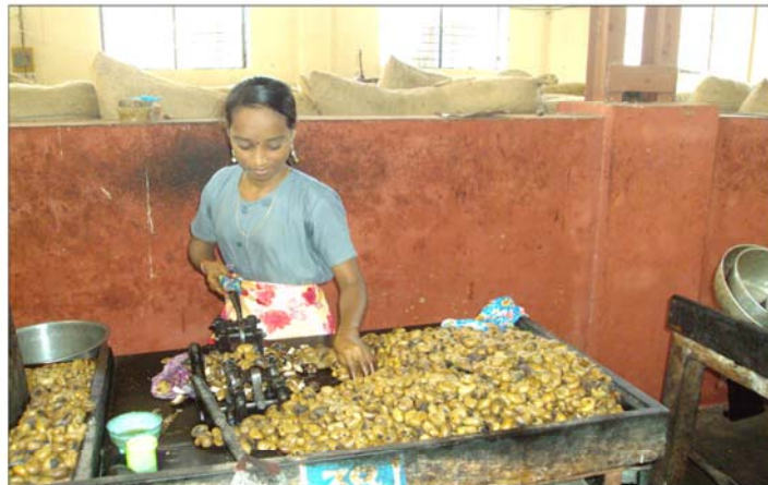
15) Cashew nut cutting process by manual.
