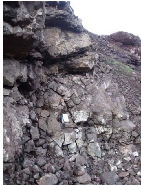
8. Block disintegration of basalt
